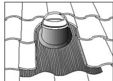
Apply High Tack sealant on the tiles that will be covered by the flashing material press the flashing material firmly to seal
